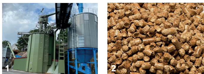
1 The picture shows the dust silo with a conveyor system that has been modified. 2 The modification of the dust recycling system has reduced the amount of dust sent to combustion and increased the degree of materials recovery.
